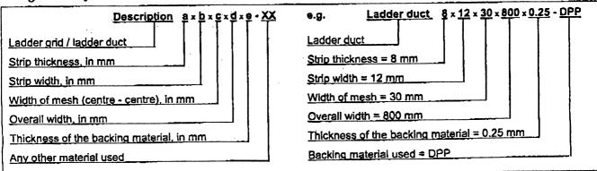
KREMPEL ladder grids and ladder ducts are made entirely from the well-known KREMPEL presspaper products. Used as the backing material are both KREMPEL transformer-grade presspaper as well as different thickness grades of
